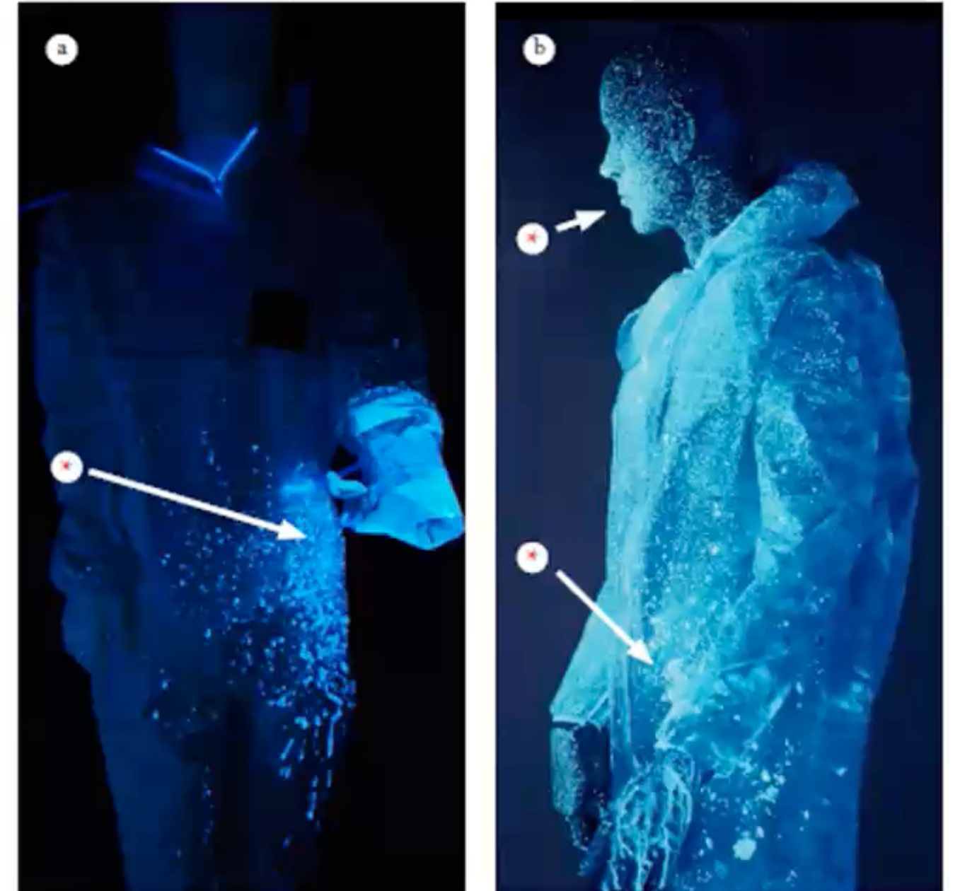
Figure 17: a and b) Photographs of MWF contamination on the torso and face (of a manikin) showing the effects of using a compressed airline and splash back onto the operator (The asterisk marks the spots / deposits on the face and arm visualised by adding a fluorescent blue dye to the MWF c
